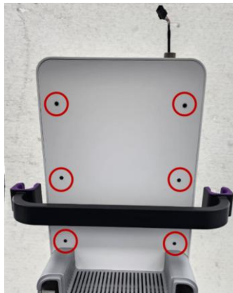
Figure 7: Remove Back Screen Cover
